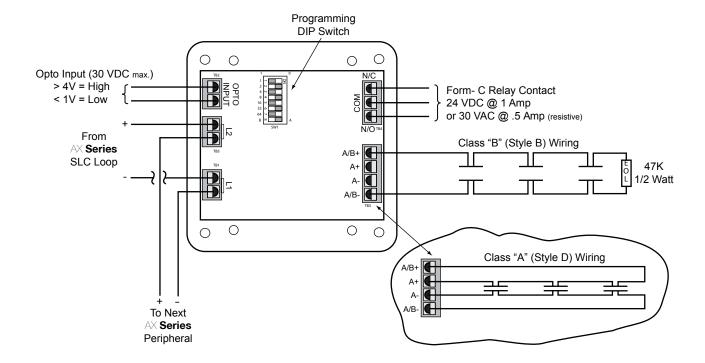
The optically isolated voltage input of the 55000-820ADV is utilized for special applications when unsupervised status monitoring of a voltage input is required (i.e. HVAC status, ancillary product status, manufacturing process equipment status, etc.).
