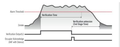
2nd Stage Verification Time started on activation of AlarmCalm button. Signal drops below alarm threshold before end of 2nd Stage Time. System returns to Normal.
