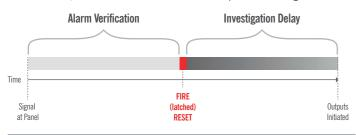
Verification and investigation comprise the two stages of complete false alarm management. Both are handled separately but configured in the same simple, powerful way using our AlarmCalm software.
