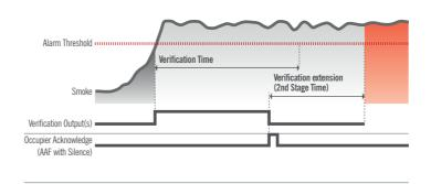
Signal remains above alarm threshold at end of 2nd Stage Time. System enters full alarm condition. The AlarmCalm button is highly flexible and easily installed and configured:
