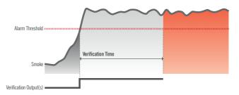
Signal not cleared, system in full fire condition at end of verification time.
